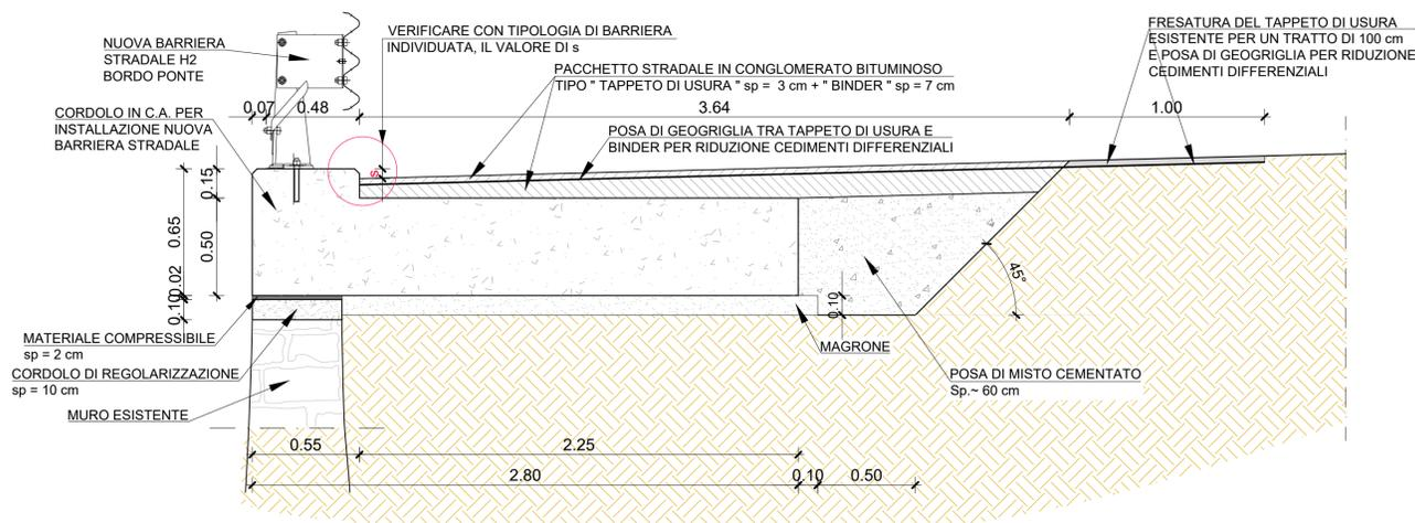
SEZIONE TIPOLOGICA BARRIERA H2 SU RILEVATO | SCALA 1:20
